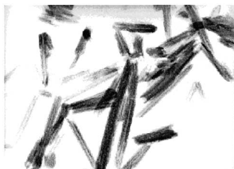
Fig. 2. TEM of typical halloysite microtubules (magnification \times 100000 ).
